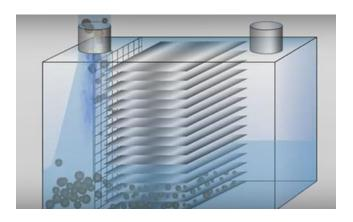
In the case of sedimentation, the amalgam particles are separated in the waste water by means of gravity. The waste water from dental units, suction tubes and sinks initially flows through a presedimentation zone in which the large particles are captured. In the next phase of the process the amalgam particles are collected in a silt chamber. Finally the smallest waterborne amalgam particles are captured in a fine sedimentation zone by means of lamellas.
